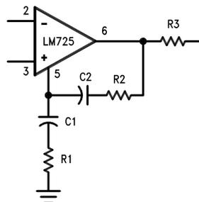
Figure 19. Frequency Compensation Circuit
