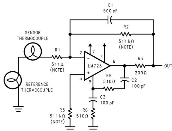
Figure 1. Thermocouple Amplifier
