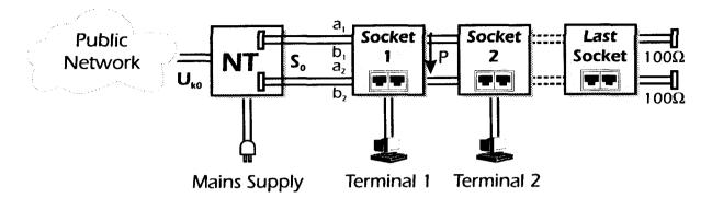
Up to 12 ISDN sockets may be installed on a single S-bus, and up to 8 terminals may be connected.
