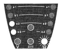
The LED display alternates between the two connections: in the above example, first a1 and b1 flash green, then a2 and b2.
