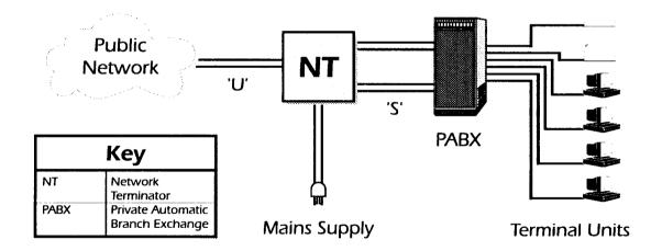
Individual units (telephone, fax, modem, etc.) are connected to the PABX.
