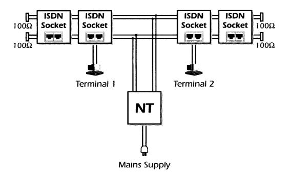
The  $100\Omega$  resistors in the NT must not be connected. The total termination resistance measured from the NT should be around  $50\Omega$  (parallel connection).
