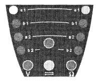
When aurora profit detects that lines are crossed, the Line LEDs for each of the crossed lines flash alternately red and green. In the example below, lines a1 and b1 are crossed.
