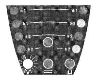
As each pair of LEDs lights up, the analogue display shows the S-bus voltage for that pair of wires.
