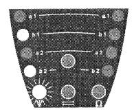
As each pair of LEDs lights up, the analogue display shows the S-bus voltage for that pair of wires. During normal operation, a voltage of 40V should be measured across a1—a2 and b1—b2.
