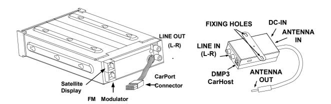
The **FM Modulator** is connected to the **DIFF** through the CarHost frame. Power supply and data communication needed for controlling the frequency happens through the RJ11 6/6 cable, which needs to be connected to the apropriate output of the CarHost. Sound signal can be connected from the line output using shielded RCA cable. The order of making the connections is irrelevant.
